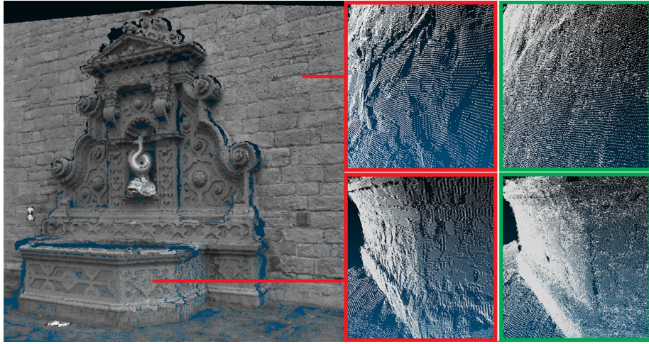
Fig. 2: Reconstruction from views 2-3 of the Fountain P11 dataset using [2] (left). Geometric artifacts are clearly visible in the closeups (middle). Whereas, the geometry of the scene is better captured with our approach (right).
